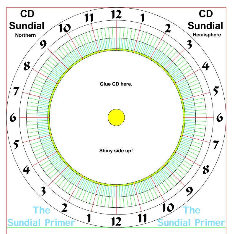
Cut along the red lines. Fold along the green line. Draw a line on the back of the dial plate parallel to the green line and 5 inches above it. This line will be 2-3/4 inches below the top of the dial plate.
