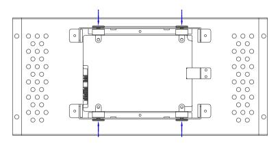
Step 5: Assembly the damper bracket
