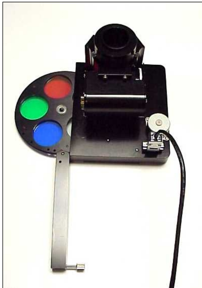
Figure 3-4. IFW with Door Open for Wheel Change (shown with TCF focuser)
