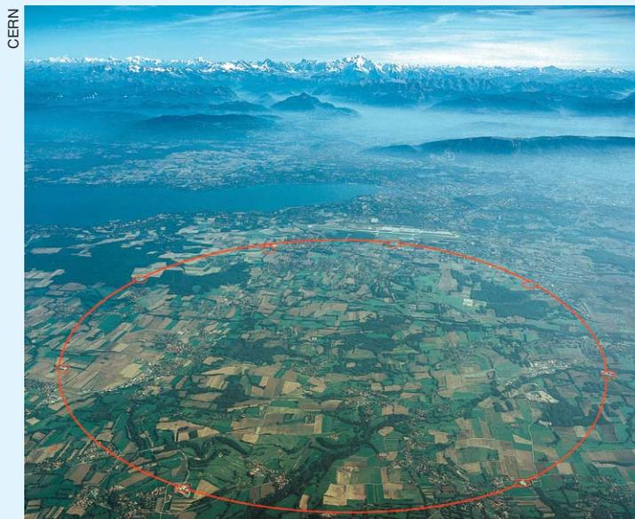
**Figure 1. The CERN laboratory** straddles the Swiss–French border near Lake Geneva. The 27-km-circumference red circle traces the underground tunnel of the lab’s Large Hadron Collider. Mont Blanc, the highest peak in the Alps, appears on the horizon.
